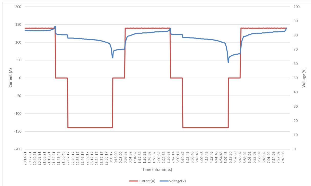
Module charge and discharge voltage/current profiles
