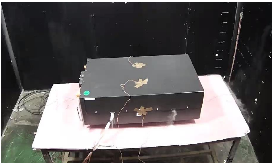
Cell vent observed
